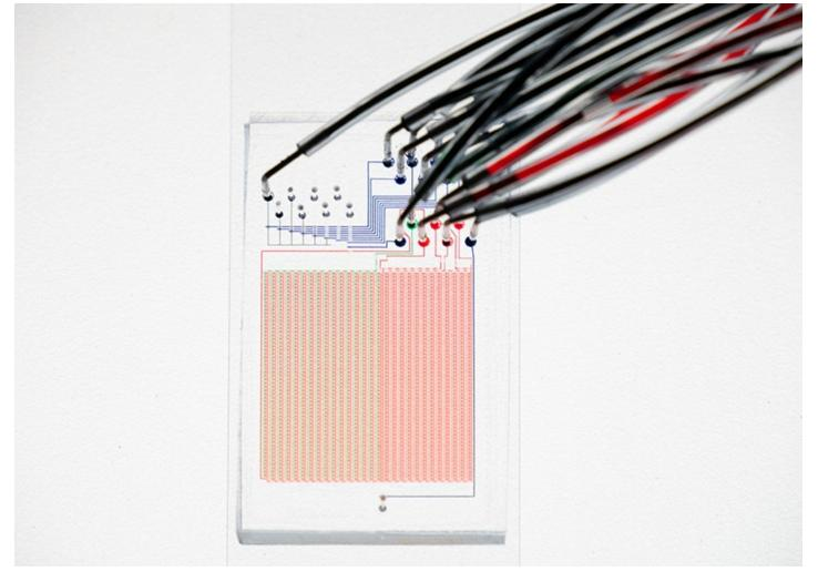
The silicone microfluidic chip has an array of 1,568 reaction chambers. Channels etched in the chip connect the chambers to control pipes attached to the top. Credit: Daniel Mokhtari
