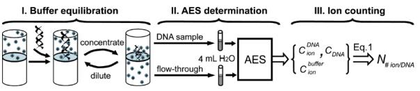
Figure 2. Scheme of the buffer equilibration-atomic emission spectroscopy (BE-AES) approach.
